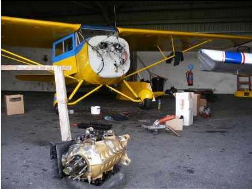
*Engine-less Ivor! Investigation of low compressions revealed a spun centre bearing, requiring a complete strip down.*
