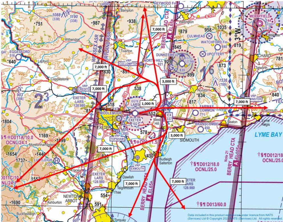
Figure 2 – Runway 08 Standard Instrument Departures (VFR Aeronautical Chart)
