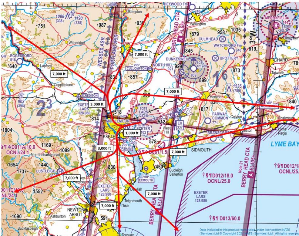
Figure 4 – Runway 26 Standard Instrument Departures (VFR Aeronautical Chart)
