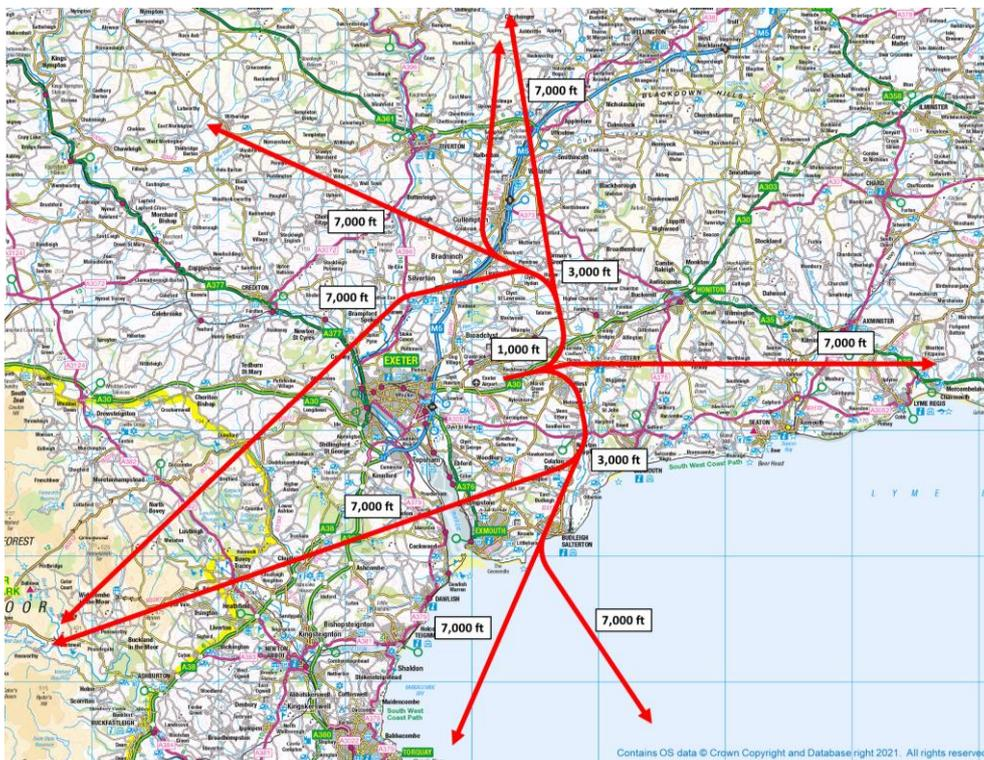
Figure 1 – Runway 08 Standard Instrument Departures (OS Mapping)
