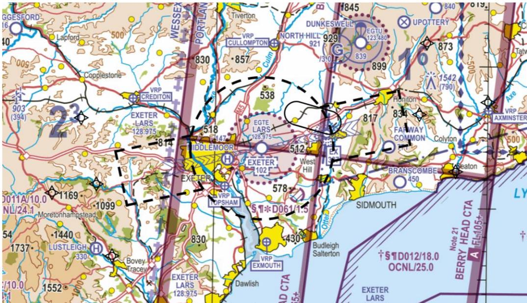
Figure 14 – 5 nm Circle with 4 nm Wide Stubs
