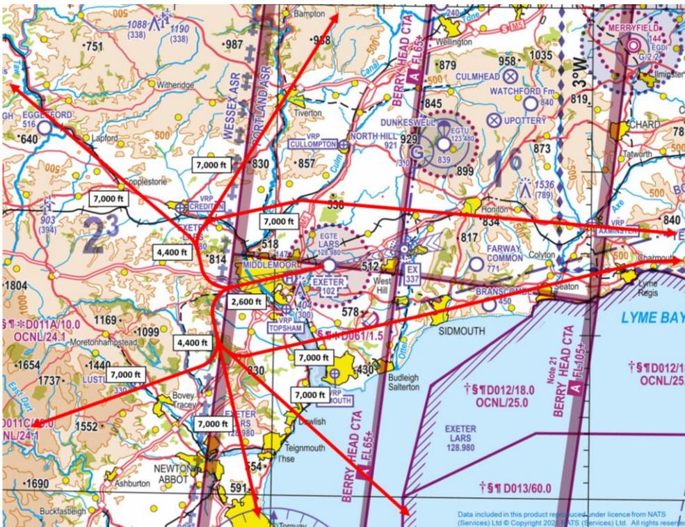
Figure 6 – Runway 26 Extended Standard Instrument Departures (VFR Aeronautical Chart)
